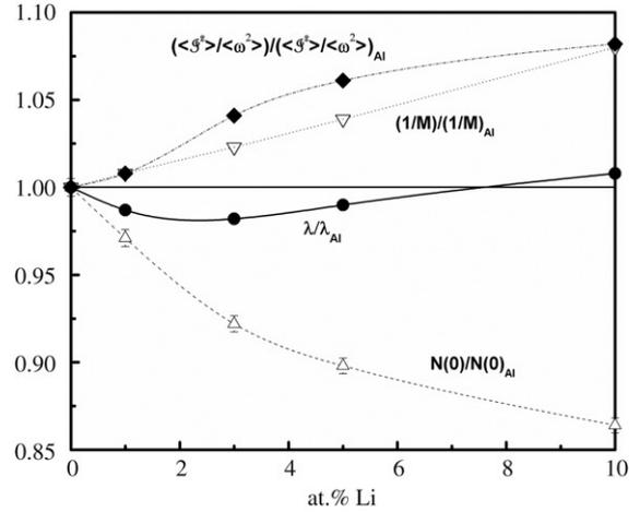
Fig. 5. Li-content dependence of normalized parameters in Eq. (4), relative to pure Al. The error bar of  $N(0)$  reflects the uncertainty in calorimetrically determined  $\gamma$ .
