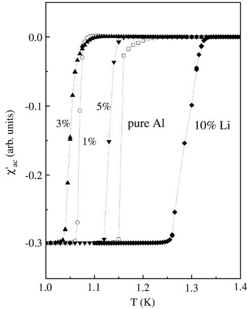
Fig. 3. Magnetic susceptibility data showing superconducting transitions.
