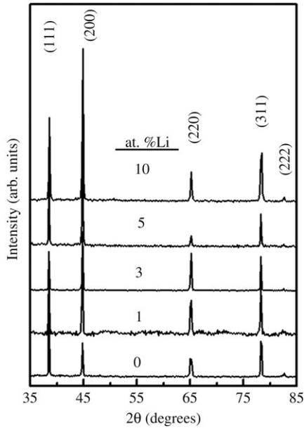
Fig. 1. X-ray diffraction patterns confirming the fcc structure in all samples.
