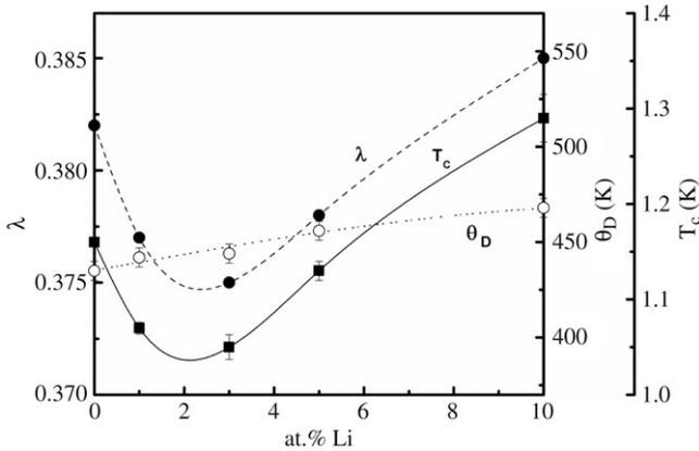
Fig. 4. Li-content dependence of  $\lambda$  calculated from experimentally derived  $T_c$  and  $\theta_D$ .
